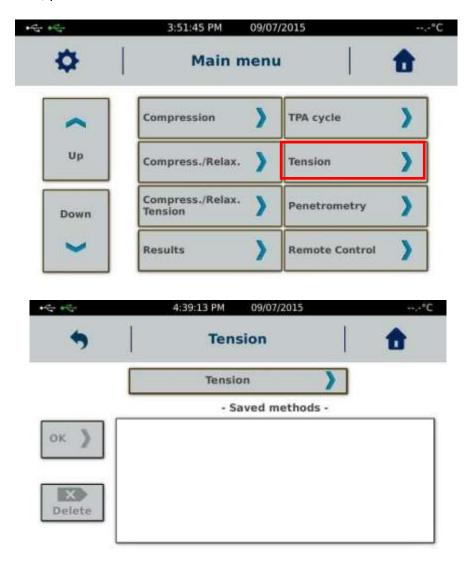
Select "Tension" to define one, creates a method or selects a method previously registered in TX-700 memory:
