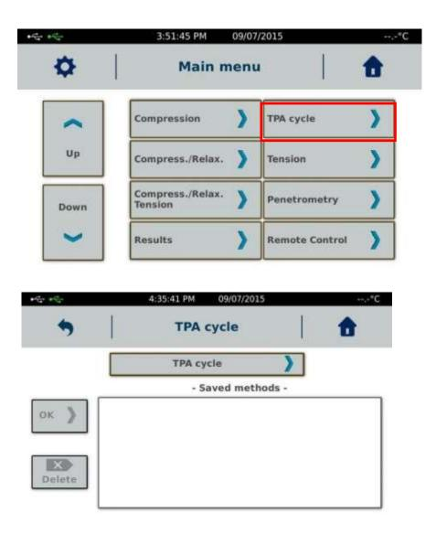
Select "TPA Cycle" to define one, create a method or select a previously saved method in the TX-700 memory:
