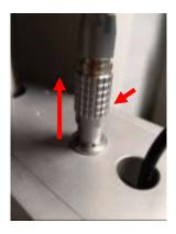
Step 2: Disconnect the connector by lifting the collar.
