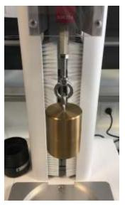
Check the measured force on the screen of the device (here 1Kg as indicated on the screen below, measured with a 50N sensor). The measured force is negative since the weight "pulls" on the sensor.
