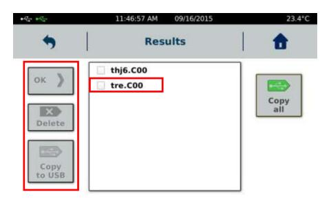
To export all data files saved in internal memory, connect a USB key at the right side of TX-700, then, one icon at the top of screen becomes green and "COPY All" is lighted up. You have just to press this icon to send the data file to USB stick.
